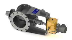
This range of dampers is designed to suit any duct size (typically Ø300mm - Ø3000mm). With SS304H construction they are resistant to corrosion, high temperature (up to 800 Deg C), and creep.
